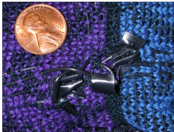
Figure 8: Taped solder bus connection
