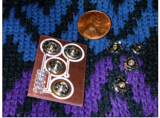
Figure 2: e-TAG and sweater snap connections
