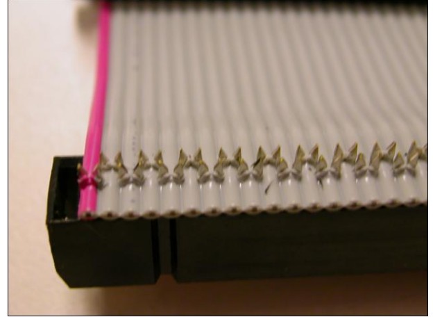
Figure 3: Ribbon cable connector with insulation displacement
